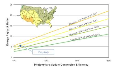
Even counting for the somewhat higher embedded energy of crystalline cells, they should, depending on where they are installed, have an overall net energy gain of 7x to 15x, and as high as 20x for some of the new ultra-high-efficiency products just coming onto the market. This compares very favorably with the corn-based Ethanol (1.3x - 2x) and soy-based biodiesel (around 3x) technologies that are getting so much attention today<sup>3</sup>.
