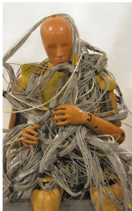
With "in-dummy DAS" (left), all the sensors, cables, and data acquisition system fit inside, eliminating the mass of sensor cables exiting a traditional test dummy (right).
