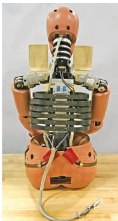
With "in-dummy DAS" (left), all the sensors, cables, and data acquisition system fit inside, eliminating the mass of sensor cables exiting a traditional test dummy (right).
