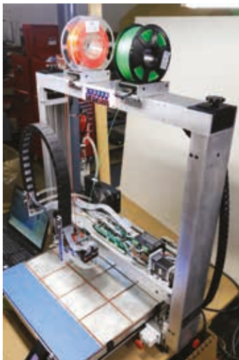
3DMonstr's T-Rex 3D series offers build volumes of up to 24 x 24 x 24".
