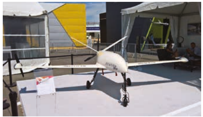
Figure 3. The ORCA drone helped verify much of the technology and construction techniques that will go into the Alice Commuter. (Image courtesy of OIDA Strategic Intelligence)
