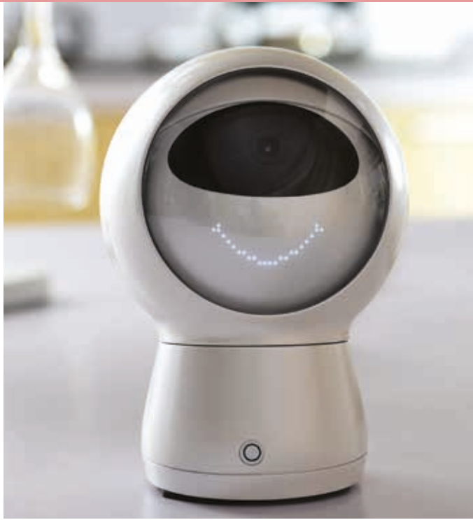
The Moorebot voice-interactive robot assistant with a warm, funny digital personality. Its AI capabilities allow it to interpret and respond to human speech, as well as infer activity and emotion from the images its camera captures. Photo: Courtesy of Moorebot.
